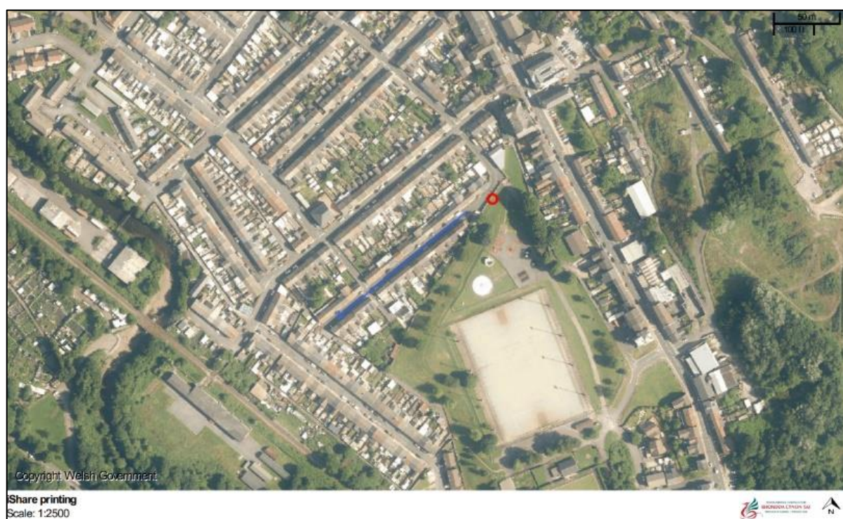
Figure 8: Location plan illustrating the location and flow path of flood water from the manhole within Pleasant Street Park
