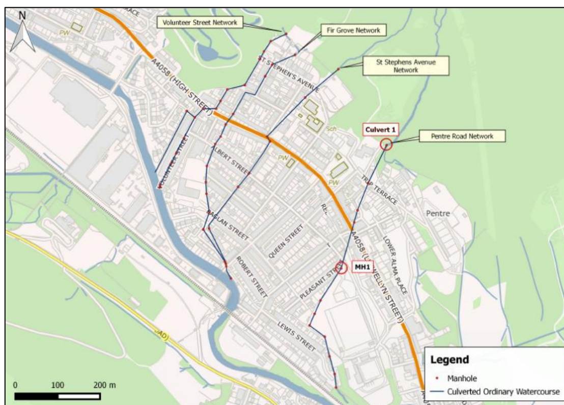
Figure 30: Ordinary watercourse structures identified as flood sources during the 2020 flood events in Pentre
